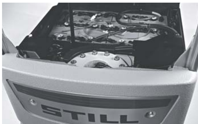
Direct access to the battery via battery compartment with a wide opening
