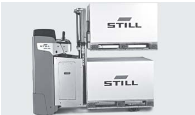
Just as safe with two pallets: use as double deck or high lift pallet truck
